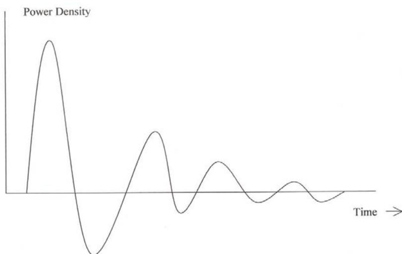
**Figure 2 - Generic Conventional EMP Transient Characteristic**
