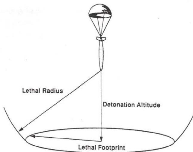
**Figure 1 - Lethal Footprint of an EMP Weapon in Relation to Altitude**
