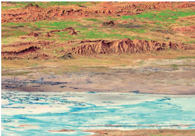
Satellite electro-optical and digital terrain elevation data can be combined to provide a virtual landscape.
