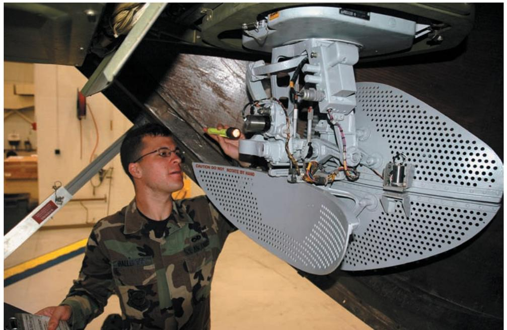
*APN-59 radar showing the mechanically switchable parabolic antenna heads (USAF).*
