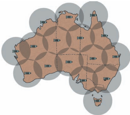
Surface coverage of airship mounted AESA radars at 60,000 feet
