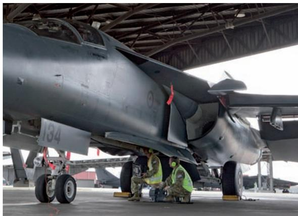
*Loading cameras into the RF-111 sensor bay*
