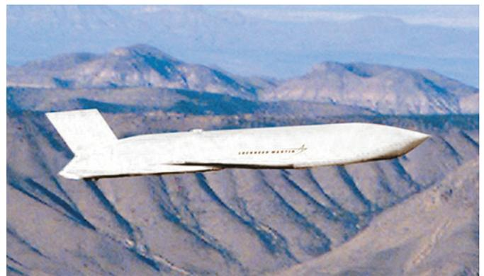
*Lockheed Martin's AGM 158 Joint Air-to-Surface Stand-off Missile (JASSM)*
