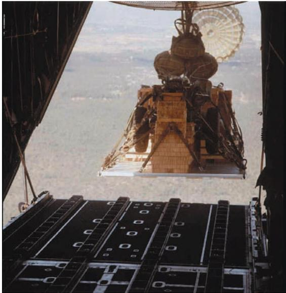
*Low velocity airdrop from a C-130 with the energy dissipater material and unopened parachutes clearly visible.*
