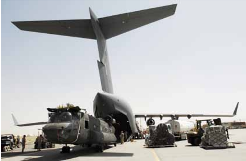
An Australian Army CH-47D Chinook helicopter being off-loaded from an Air Force C-17A Globemaster III at an airfield in the Middle East.
