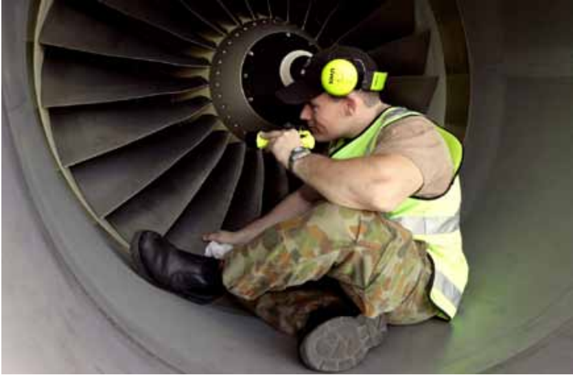
An aircraft technician with No 2 Squadron inspects the compressor blades of a Wedgetail AEW&C aircraft engine at RAAF Base Tindal during Exercise TALISMAN SABRE 2011.
