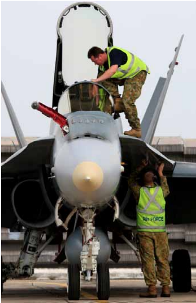
Technicians from No 3 Squadron begin to prepare for an engine run after a fuel tank change during Exercise BERSAMA PADU 2010.
