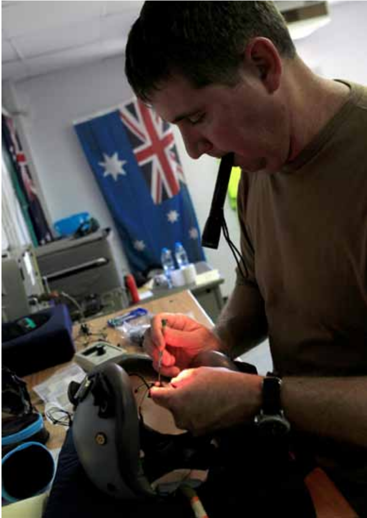
An Aircraft Life Support Fitter with No 77 Squadron, makes repairs to the main earpiece of a pilot's helmet during Exercise THAI BOOMERANG 2011.
