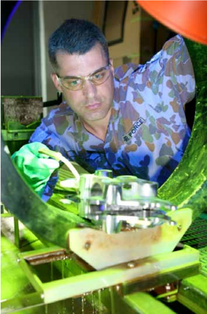
A Technician performs a magnetic particle inspection of a Hornet armament extractor housing under an ultraviolet light.
