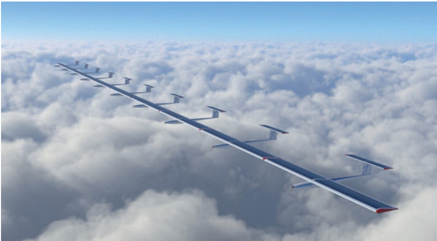
Figure 11. AlphaLink proposed a design for individually launched air vehicles to fly into a formation and autonomously connect into a single pseudosatellite 39
