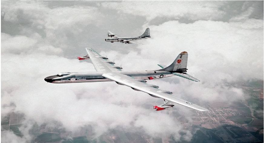
Figure 1: NB-36H Peacemaker experimental nuclear propelled aircraft 18
