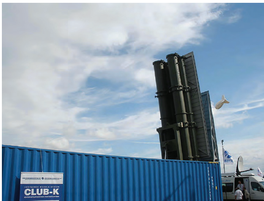
Figure 6 A missile launch system concealed in a shipping container 54
