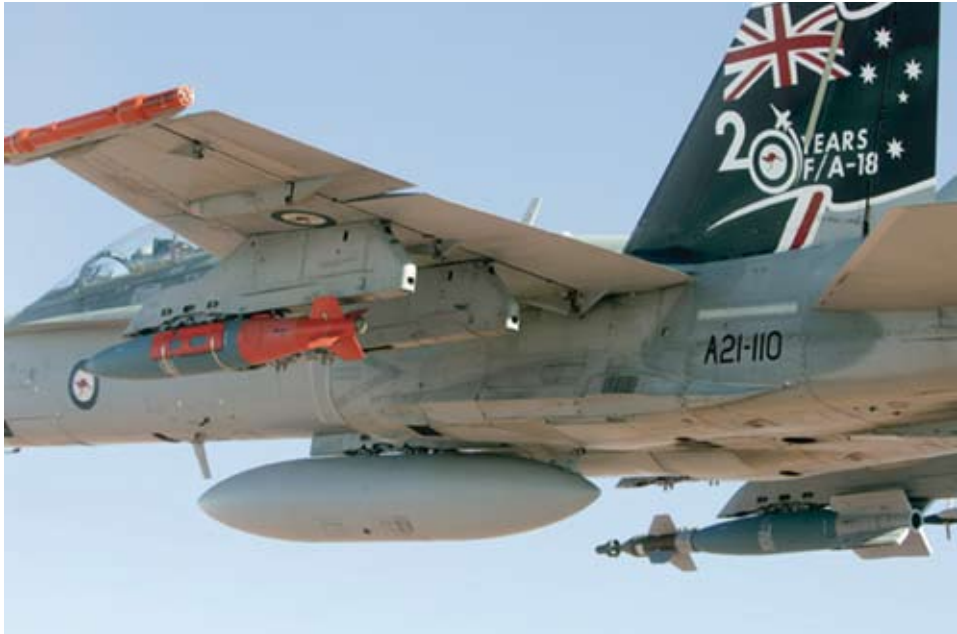
A RAAF F/A-18 Hornet armed with a GBU-32 (1000 lb JDAM) and a GBU-11 (1000 lb laser-guided bomb), and with a Time/Space Position Information pod on the wing tip during Developmental Test and Evaluation at Woomera.
