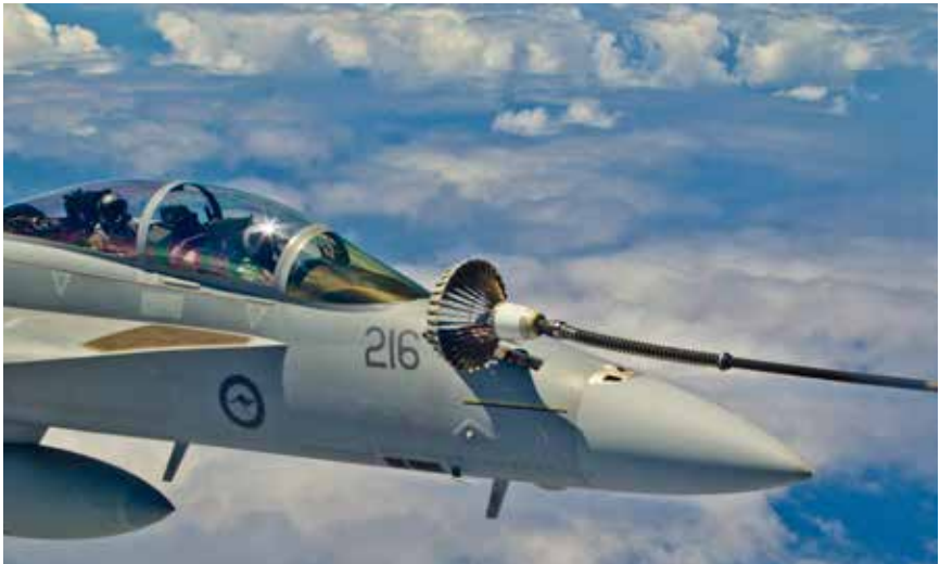
F/A-18 Super Hornet during air-to-air refuelling with a KC-30A Multi-Role Tanker Transport (Pathfinder #231)
