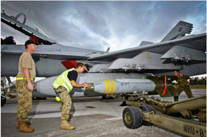
Armament Technicians loading a Guided Bomb Unit - 24 onto an F/A-18F Super Hornet. (Pathfinder #229)
