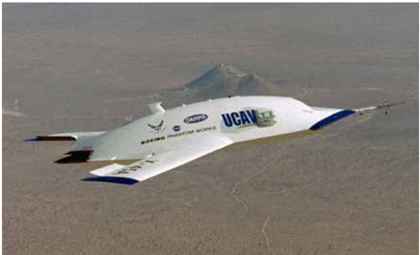
J-UCAS Boeing X-45A UCAV technology demonstrator (Source: NASA/Dryden Flight Research Center/Jim Ross, Pathfinder #223)
