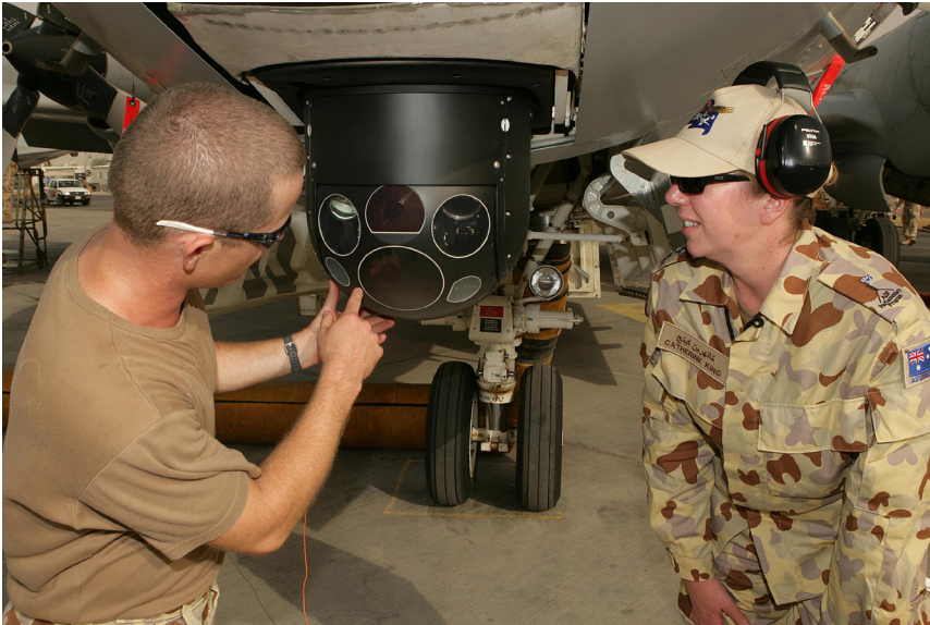
The Star Safire camera fitted to the AP-3C Orion undergoing inspection. The capable and versatile camera is an important component of the Orion's overland ISR capability. (Pathfinder #275)
