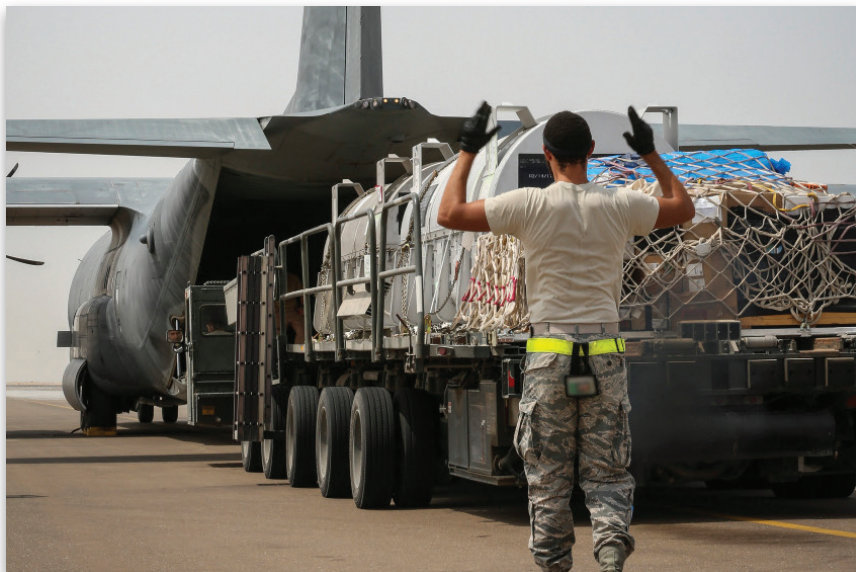
A USAF member guides a Truck Aircraft Loading and Unloading vehicle (TALU) (Pathfinder #299)
