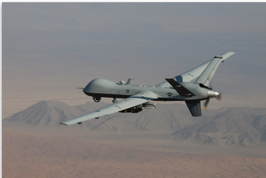
An MQ-9 Reaper over southern Afghanistan, armed with GBU-12 Paveway II laser guided munitions and AGM-114 Hellfire missiles (Photo: US Air Force). (Pathfinder #315)
