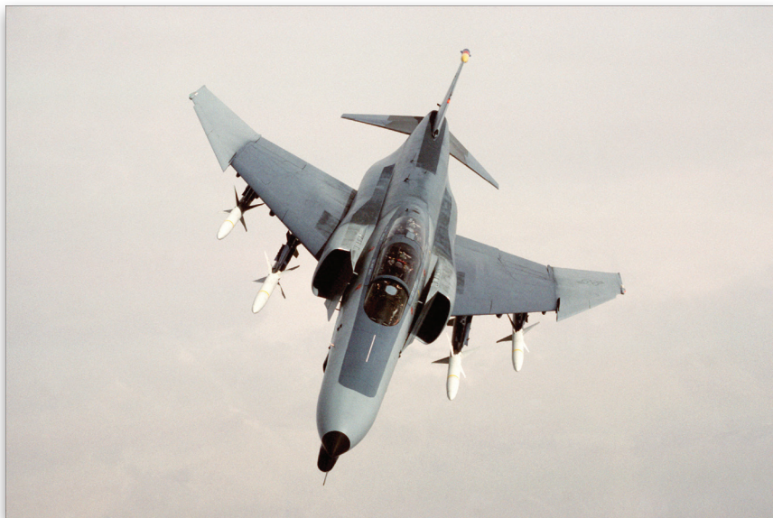
An air-to-air front view of an F-4G Wild Weasel Phantom II aircraft. The aircraft is armed with four AGM-88 high-speed anti-radiation missile (HARM) missiles (Pathfinder #339)
