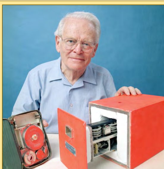
Black box flight recorder.
