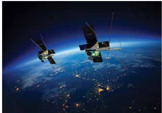
Figure 1. M2 is a twin-satellite mission. Both satellites are equipped with advanced radios and telescopes for maritime surveillance demonstrations, as well as inter-satellite communications and a number of science experiments.
