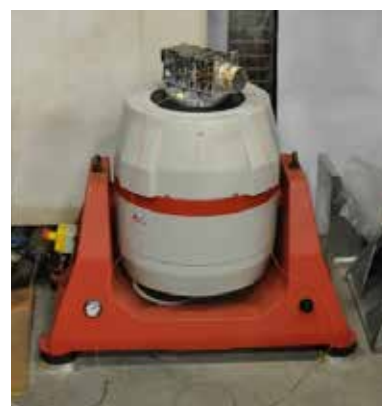
Figure 1. BMM primary HF Payload mounted to B&K table for vibration testing (left) and vibration results in the X-axis (right). The green line represents the vibration profile applied to the payload. The orange line indicates the response of the control accelerometer attached to the base plate. The blue line represents the X-axis acceleration PSD. Shaker table, right.
