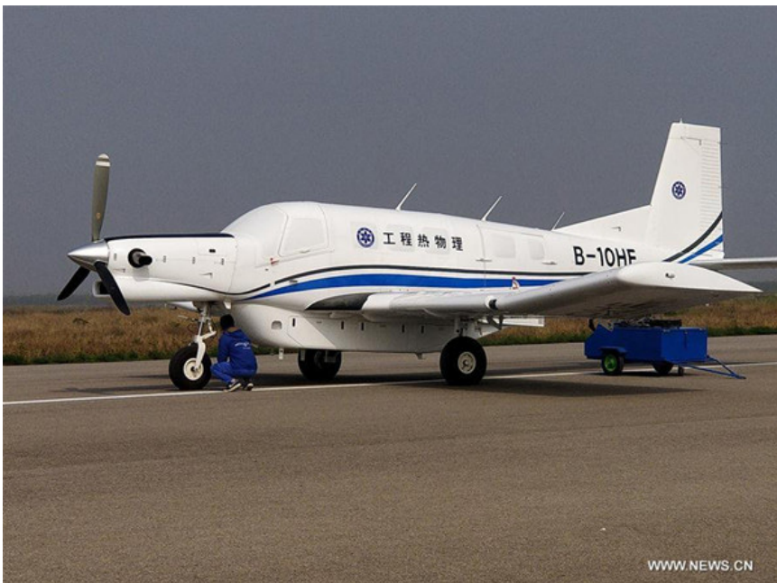
Figure 2. Chinese AT200 modified UAS cargo aircraft.
