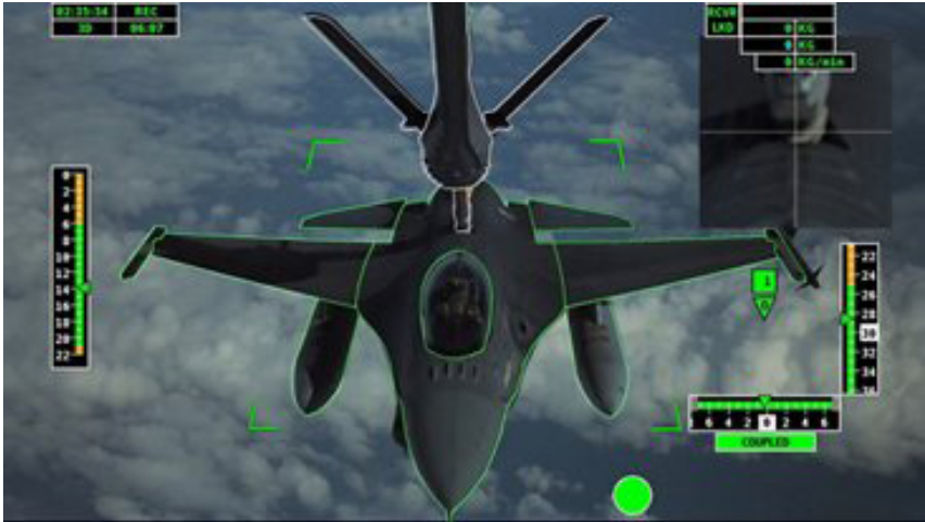
Figure 9. Detection of receiver aircraft in Airbus' fully automated A3R system.
