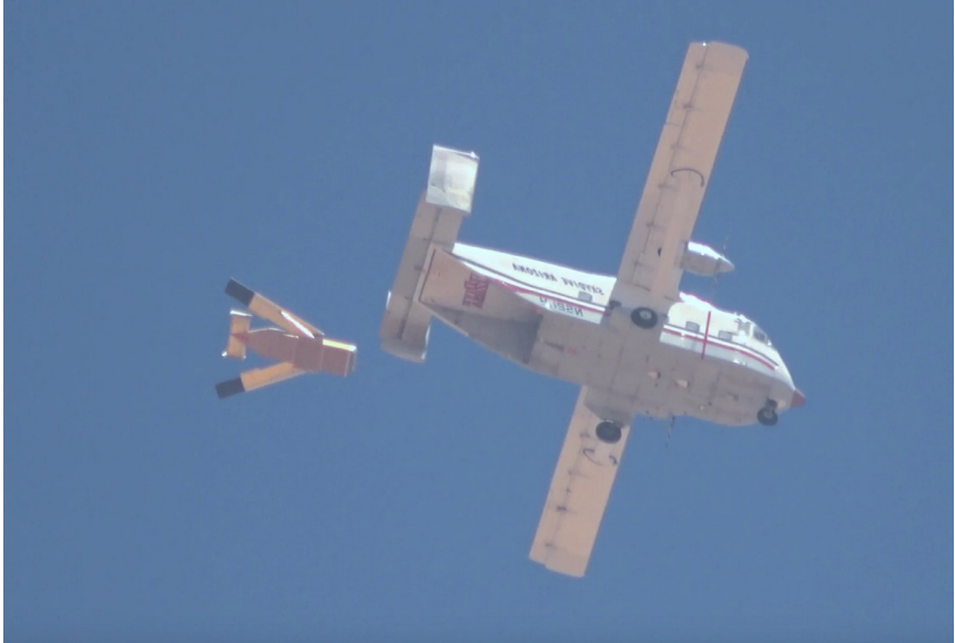
Figure 7. Logistic Gliders Inc. very low cost TACAD (TACTical Air Delivery) glider. Source: Ackerman (2019).
