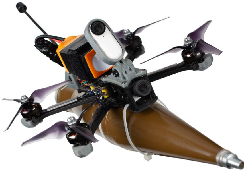
Figure 2. First Person View (FPV) drone carrying an anti-tank warhead (Source: Shutterstock ).
